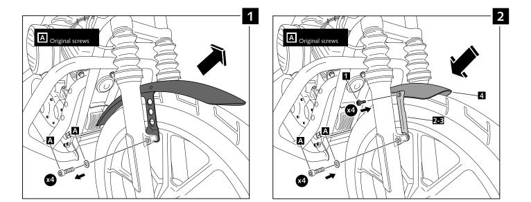
It would be convinient to re-tight the front fender screws, specially the ones that are fixed to the motorcycle, whenever you maintain the vehicle. **Thanks for your attention.**
