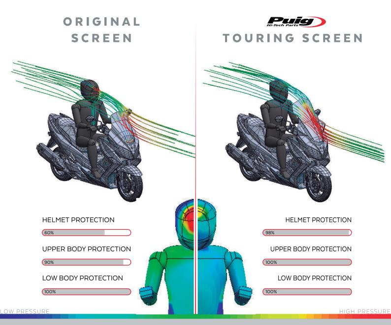
TOTAL DISSIPATED PRESSURE WITH PUIG SCREEN IS EQUIVALENT TO 2.7 Kg
