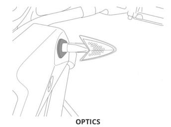
Hides the gap that leaves the OEM turn signal when it is replaced
