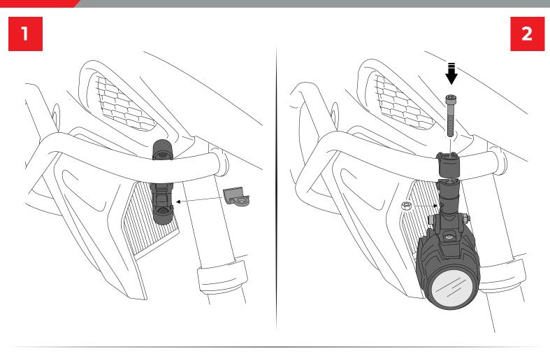
FOR THE ASSEMBLY OF THE AUXILIARY LIGHTS IN THE MOTOPLASTIC DEFENSES USE ONLY ONE OF THE 2 COARS THAT BRING THE SUPPORT AND ALLEN M6x50 SCREW
