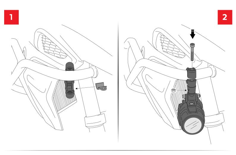
FOR THE ASSEMBLY OF THE AUXILIARY LIGHTS IN THE MOTOPLASTIC DEFENSES USE ONLY ONE OF THE 2 COARS THAT BRING THE SUPPORT AND ALLEN M6x50 SCREW
