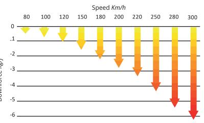
The Downforce that the spoilers generates raises potentially as the speed increases, at 300 km/h we get 6,3 Kg/f.
