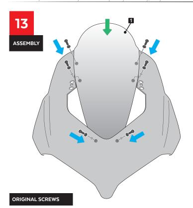
IN ORDER TO FINISH THE ASSEMBLY OF THE FAIRING, PLACE THE SCREWS BACK ON ACCORDING TO DRAWINGS 11 TO 1.
