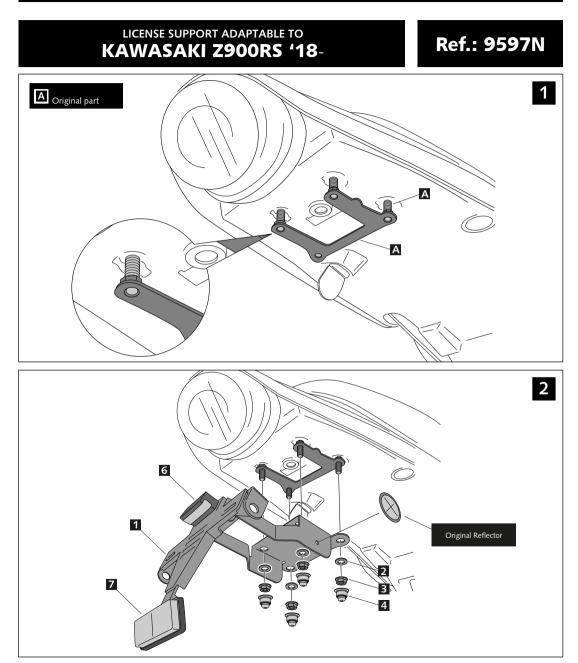
It would be convinient to re-tight the licence support screws, specially the ones that are fixed to the motorcy-cle, whenever you maintain the vehicle.
