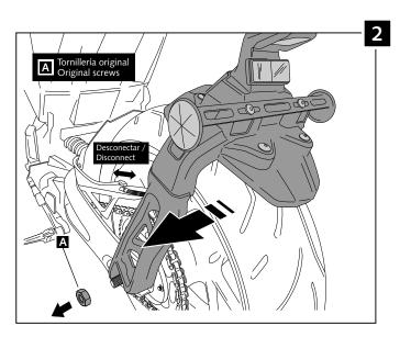
It would be convinient to re-tight the licence support screws, specially the ones that are fixed to the motorcycle, whenever you maintain the vehicle.
