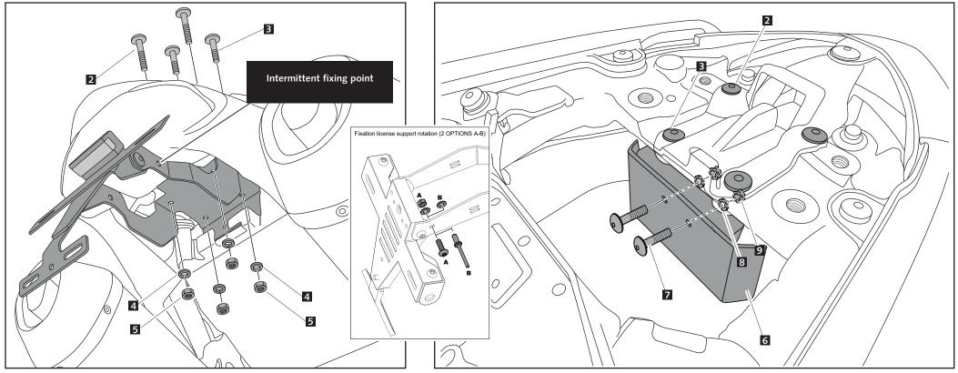
It would be convinient to re-tight the licence support screws, specially the ones that are fixed to the motorcycle, whenever you maintain the vehicle.
