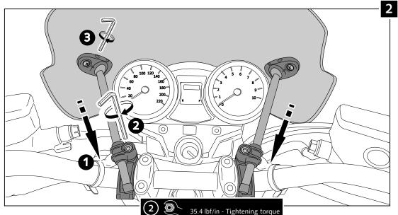
**IMPORTANT:** On some motorcycle models it may be necessary to cut the rods to avoid them touch the gas tank when turning the handlebar.
