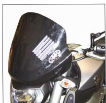
It would be convinient to re-tight the windshield screws, specially the ones that are fixed to the motorcycle, whenever you maintain the vehicle.
