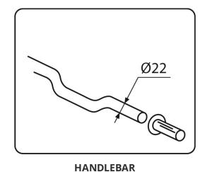
Suitable for handlebars of diameter 22mm.
