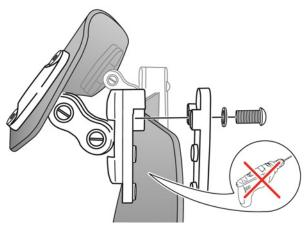
Suitable for screen thicknesses between 3 and 5mm. It is not necessary to pierce the dome to hold the visor.
