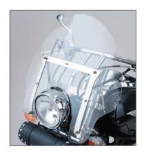
It would be convinient to re-tight the windshield screws, specially the ones that are fixed to the motorcycle, whenever you maintain the vehicle.
