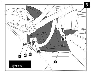
It would be convinient to re-tight the chain cover screws, specially the ones that are fixed to the motorcycle, whenever you maintain the vehicle.
