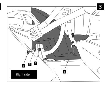
It would be convinient to re-tight the chain cover screws, specially the ones that are fixed to the motorcycle, whenever you maintain the vehicle.
