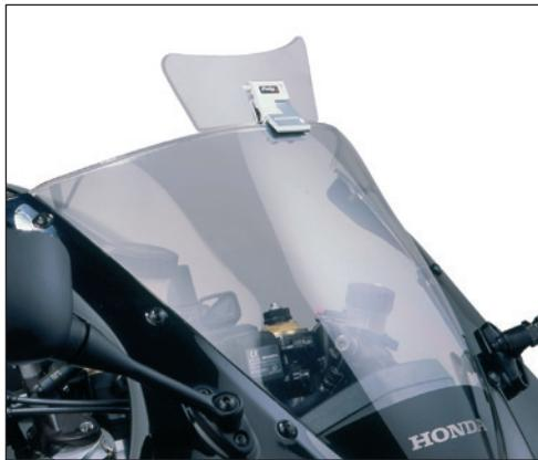
It would be convenient to re-tight the windshield screws, specially the ones that are fixed to the motorcycle, whenever you maintain the vehicle.
