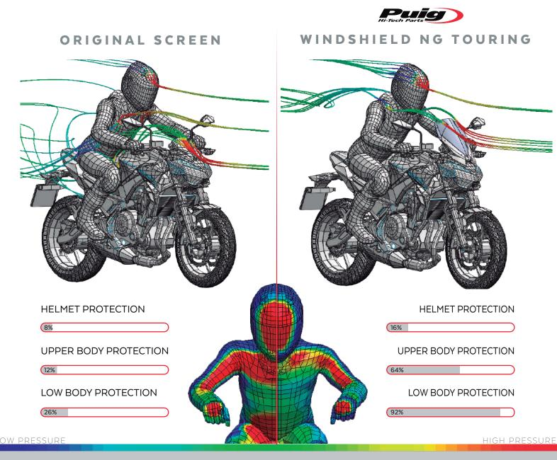
TOTAL DISSIPATED PRESSURE WITH PUIG SCREEN IS EQUIVALENT TO 3,6 Kg
