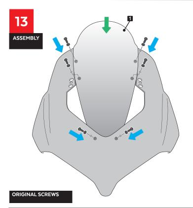
IN ORDER TO FINISH THE ASSEMBLY OF THE FAIRING, PLACE THE SCREWS BACK ON ACCORDING TO DRAWINGS 11 TO 1.
