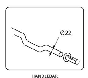
Suitable for handlebars of diameter 22mm.
