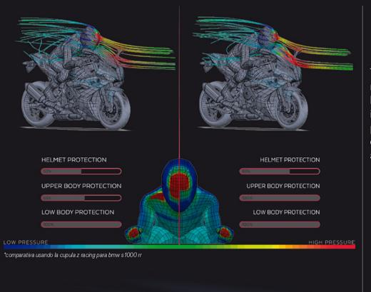
The Z-Racing screens are designed to be aerodynamically more efficient than the original screens of each motorcycle, being tested in the **virtual wind tunnel** to ensure that they improve the aerodynamic coefficient (Cx) and the aerodynamic protection of the rider thanks to its double bubble height design, deflecting the wind that would affect your helmet and upper torso.
