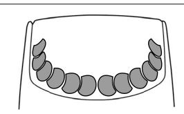
Attach a few stick-fit pads to the Hugger Extension in area shown to create a gasket.
