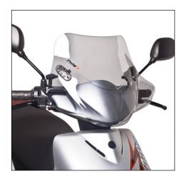
It would be convinient to re-tight the windshield screws, specially the ones that are fixed to the motorcycle, whenever you maintain the vehicle.
