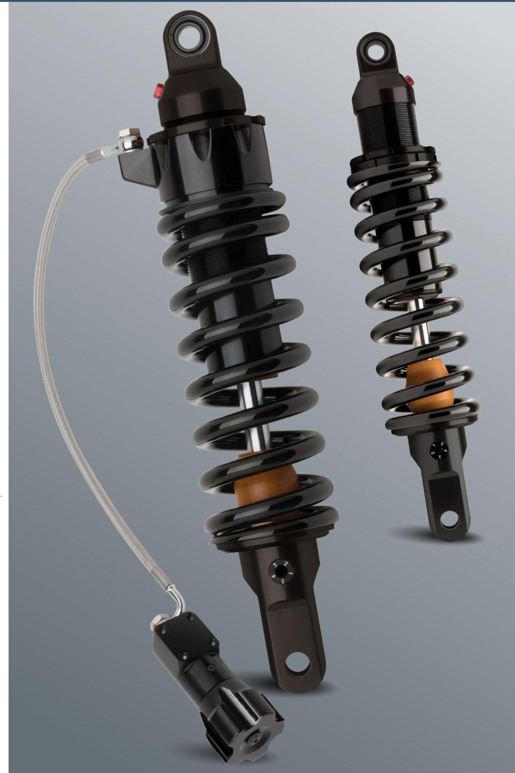
The 465 Series represents state of the art high pressure gas monotube shock design. It utilizes a large 46mm bore and deflective disc piston for precise damping. The beefy 16mm hard chrome shaft rides on custom viton seals for low friction and leak free life. Choose the R.A.P. (Remote Adjustable Preload) version that has a 5 position rebound adjuster that sets it up to perfectly match your bike, weight and riding style. Built in the USA.
