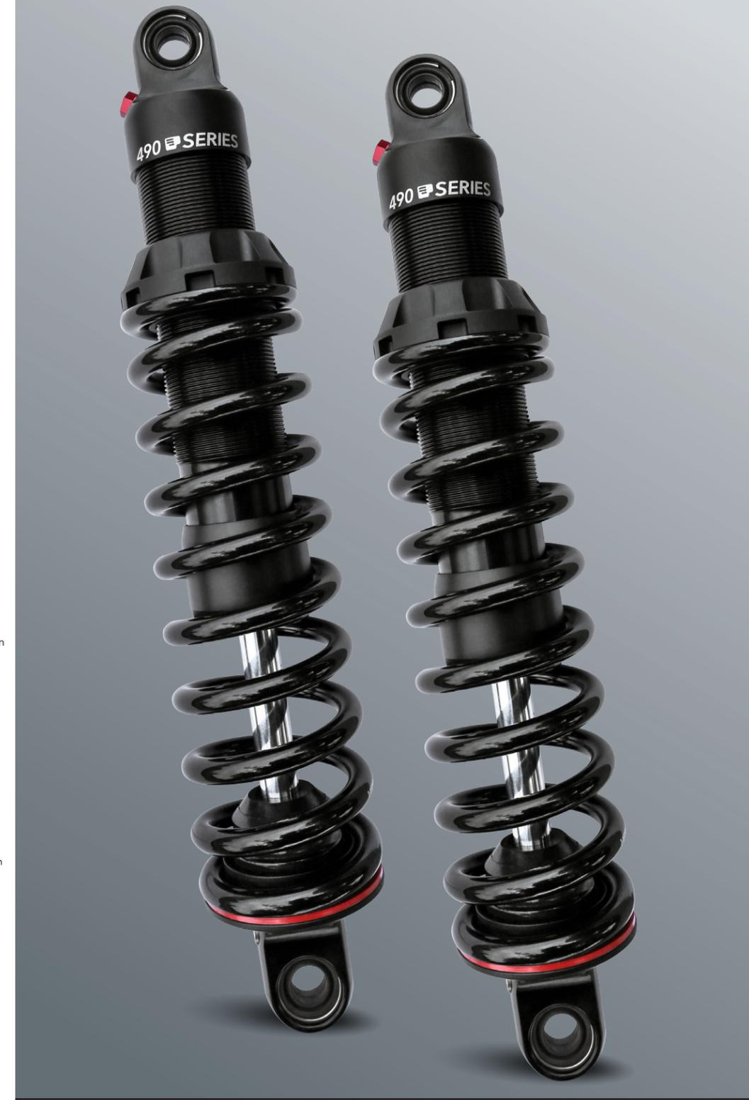
A true sport performance shock at heart with a competitive price tag, the new 490 Sport Series Shocks feature a high-pressure monotube with deflective disc damping technology, hand threaded preload and a rebound adjustment to dial in the ride. An engineered jounce bumper with a built-in metal cup also help smooth out and control bottoming. From pounding the pavement around town to hammering around the tarmac on your next race day, the 490 is the perfect choice for your performance demand!
