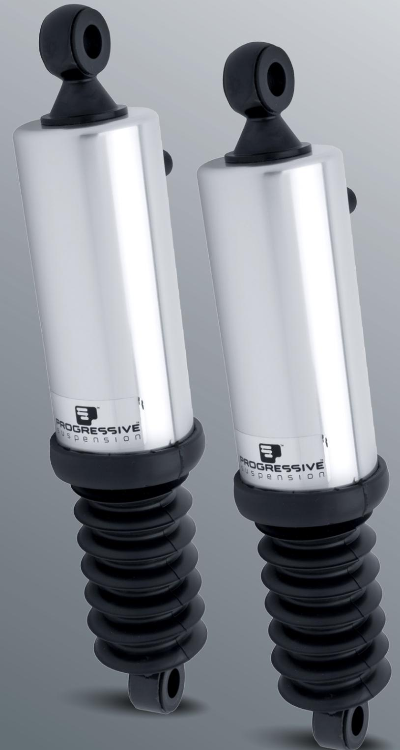
The Original Air Shock from Progressive Suspension features a machined aluminum air chamber for perfect sealing surfaces, heavy duty springs, air adjustability and velocity sensitive, multi-stage valving. The 416 Series is the perfect choice for the touring rider who carries a varied load. An optional adapter kit is available for most touring bikes to tap into the stock air fill system (fill valve or air compressor). Built in the USA.
