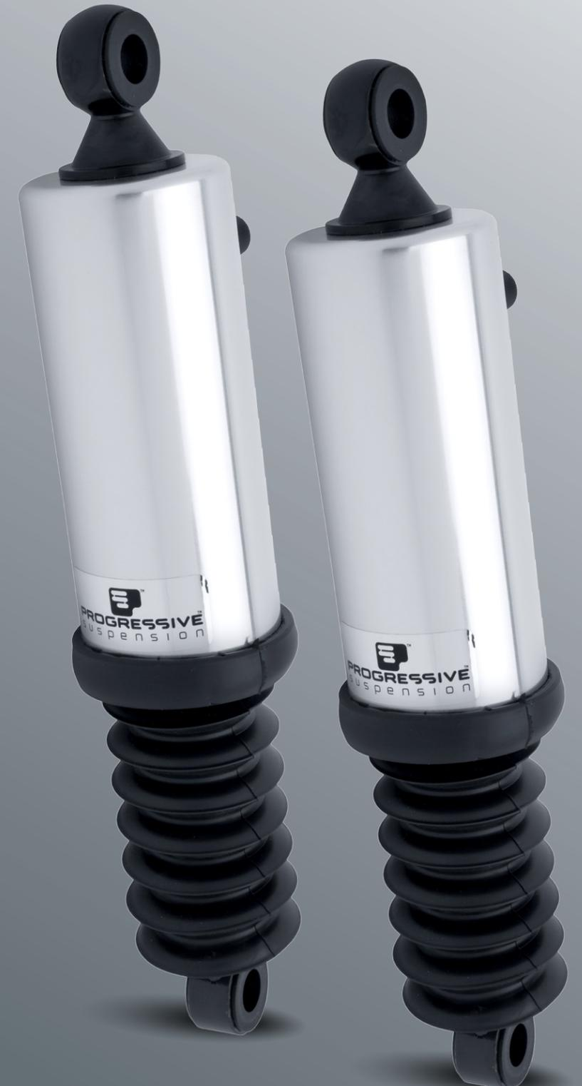
By combining a machined aluminum air chamber, velocity sensitive, multi-stage valving and an internal progressive rate coil spring, we've once again elevated air suspension to a new level. The clean and simple, full chrome body mounts to all late model touring bikes and is powered by a clever compressor unit that uses a hook and loop style fastener to mount into the back of a saddlebag.
