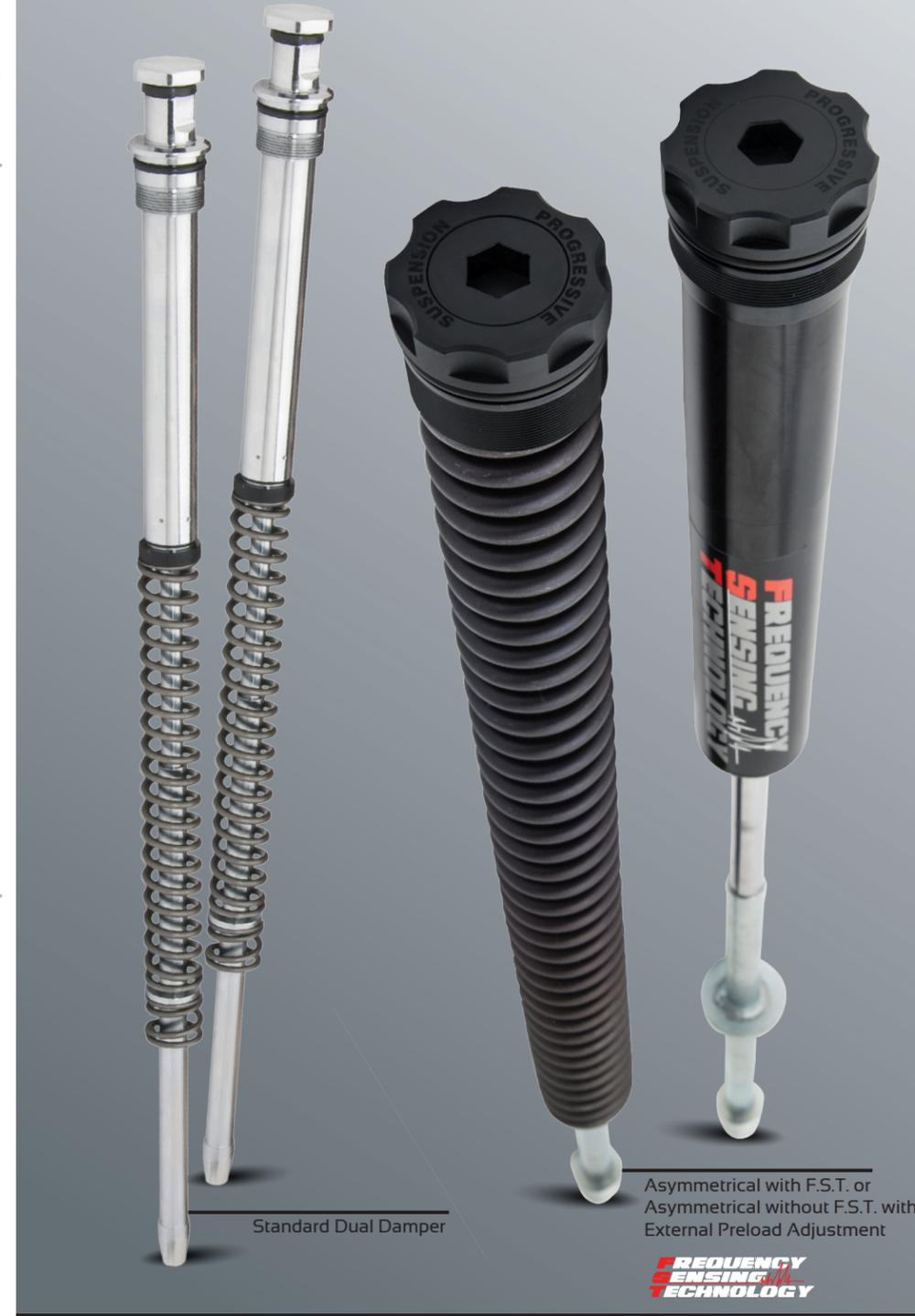
The F.S.T. Monotube Kit is a true high performance front suspension. Progressive Suspension has combined their road smoothing Frequency Sensing Technology (F.S.T.) damper with a progressive rate spring to create a state of the art fork cartridge kit.
