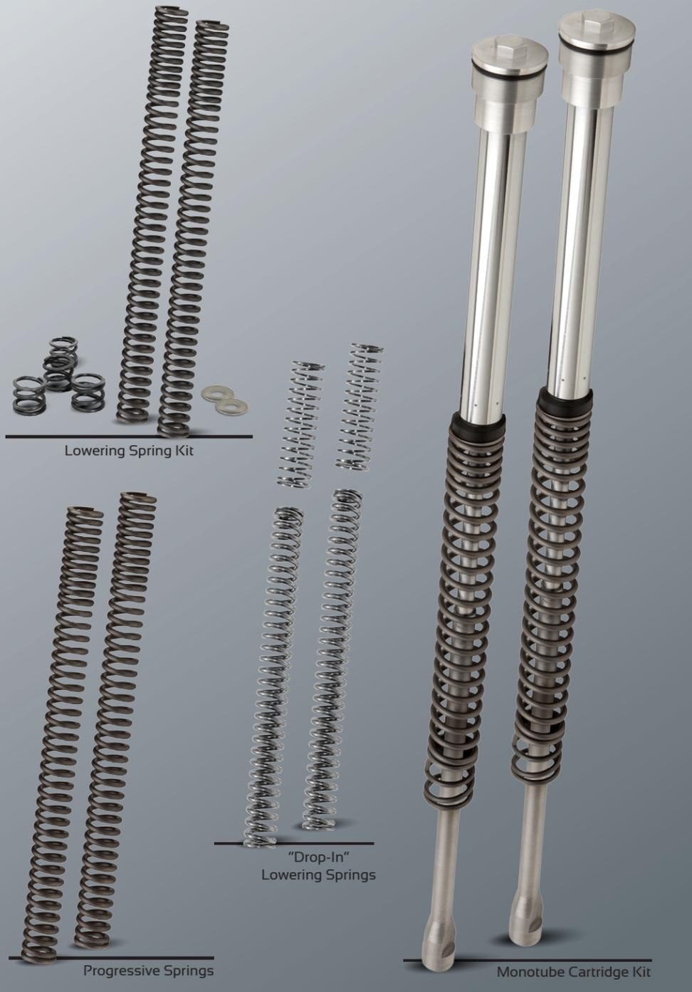
Progressive Suspension's state of the art **Monotube Fork Cartridge Kit** is designed for the performance oriented rider who demands both handling and ride quality. The kit replaces the sloppy open bath internals of the stock fork with a set of gas charged monotube dampers and custom tuned fork springs. Monotube style damping improves ride comfort, resistance to front brake dive as well as improving front end stability, cornering and bottoming control.
