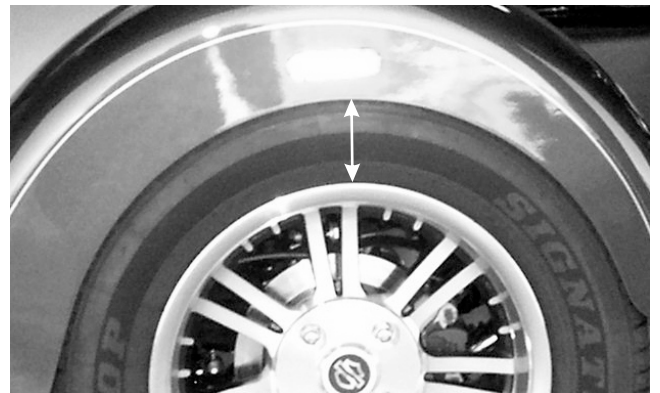
Figure 4 The difference in measurements between the top of the rim and the fender with the suspension fully extended and then with rider(s) on the bike is your Ride Sag. This difference should be .80" - 1.2" for maximum ride comfort.
