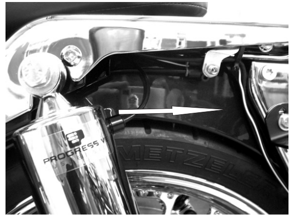
Photo 2 Install shocks so air fittings points rearward.
