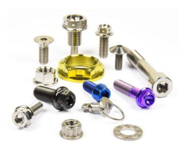
Made from aircraft grade titanium 6AL-4V (grade 5), the outstanding benefits are that we roll the threads to produce greater fatigue strength and reduce galling. These bolts are in excess of 120,000psi ultimate tensile strength, suitable to replace both Grade 5 and Grade 8 steel bolts. We offer Race Spec drilled Flanged Hex Head Bolts, Flanged Hex Head, Tapered Socket Cap, Countersunk Bolts, Dome Head Bolts, Nuts and Washers – from 3mm to 12mm.
