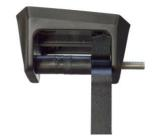
STEP 5: At this time go back and check the torque of all fasteners. All fasteners may need to be retightened after the first ride. Check the tightness of the bracket and handguard before each ride.
