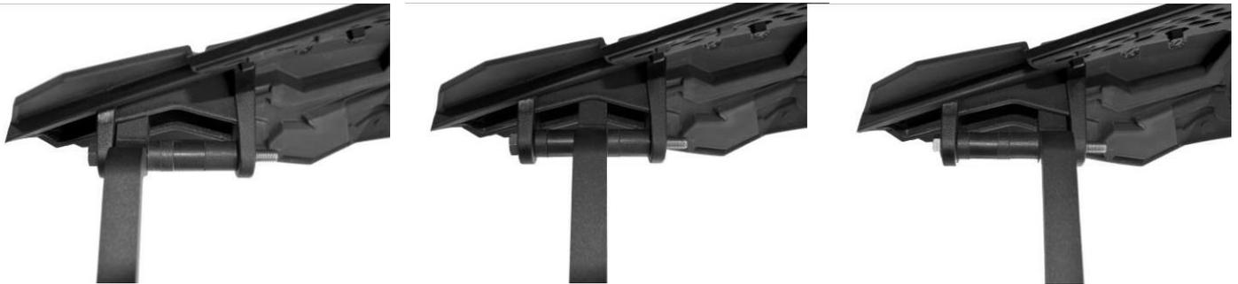
**STEP 5:** At this time go back and check the torque of all fasteners. All fasteners may need to be retightened after the first ride. Check the tightness of the bracket and handguard before each ride.
