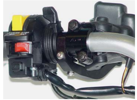
Right side view of ATV, bracket is positioned under brake lever and angles toward center.
