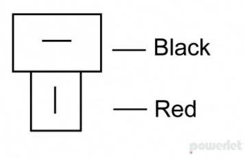
Uses 1/4" spade terminals in a "T" configuration. Used by Powrelet and some vehicle manufacturers like Victory, Aprilia and Triumph.
