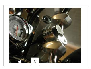
STEP #5 – Do NOT allow the harness to directly contact the motor or exhaust.
