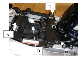
**STEP #3** – Connect the two white "T" connectors to the back of the sockets[A]. Slide on both straight rubber boots over the back of the sockets. Do this before attaching the bracket; it requires special monkey fingers after the bracket is attached.
