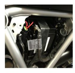
STEP #2 – Stretch out the wiring harness. Grab the rubber boot (covering the white t-connector) end of the harness and start routing the harness from the right side near the battery to the left side passenger foot peg. Next remove the negative battery connection, followed by the positive battery connection. Connect the red & black wire as follows:
