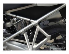
STEP #4 — Attach the white connector from the harness to the white connector on the bracket. Cover connection with rubber boot. Install the fuse in the fuse-holder. Apply either dielectric grease or Vaseline to the terminals. Connect the red wire to the positive terminal & the black wire to the negative terminal. Use a voltmeter to check if the polarity is correct. The center terminal is positive and the outer ring is negative.
