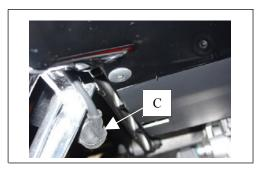
STEP #3 – Attach the bracket to the front rearset-mounting lug. The wiring coming from the socket should route towards the rear of the bike[C]. The rearset needs to be removed completely. The supplied spacer must be placed in the rear to maintain proper alignment. Reinstall the rearset with the bracket & spacer sandwiched between the rearset & the frame. Re-use the stock bolts.
