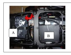
STEP #2 – Stretch out the wiring harness. Grab the white connector end of the harness and start routing the harness by looping the wires down through the gap between the frame member and the battery compartment plastic. Next remove the negative battery connection, followed by the positive battery connection. Slip the red wire under the red battery boot[A]. You may need to trim the red boot to accommodate the added wire. Connect the red & black wire as follows:
