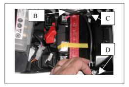
**STEP #3** – Install the fuse in the fuse-holder. Next attach the spade connectors to the socket. The center terminal of the Powerlet socket is plus and the outer ring is negative (see dwg below). The boot on the back of the socket are oriented so the wiring harness will route straight up from the socket, hiding it under the tail fairing.
