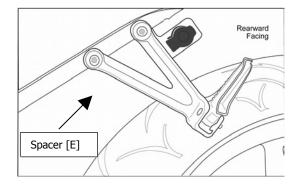
Many times the exhaust is hanging from the rearset and this can be heavier than expected. If your exhaust is hanging from the rearset, loosen both rearset bolts but do not remove them from the tail section sub-frame. By removing only one bolt at a time the weight of the exhaust will hang on the installed bolt. The bracket fits between the sub-frame and rearset and the supplied spacer [E] must be placed between the sub-frame and other rearset mounting point to maintain proper alignment.
