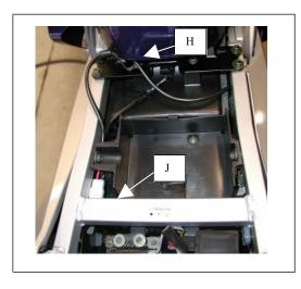
STEP #3 – Adjust the slack in each section, tighten ty-wraps.
