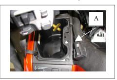
**GL1800 (2006-Present)** – Drill on dimple in the plastic. Also for step #4 you will find the red connector located inside rubber boot.
