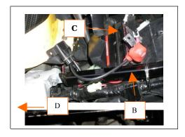
STEP #3 – Install the fuse in the fuse-holder. Attach the wires to the socket. The center terminal is plus and the outer ring is negative (see dwg below). Apply either dielectric grease or Vaseline to the spade terminals. Connect the red wire to the positive spade terminal & the black wire to the negative spade terminal. Use a voltmeter to check if the polarity is correct.
