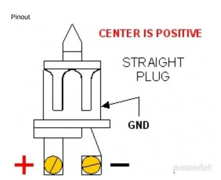
Powersport Standard Connectors are fully DIN ISO standard compliant. Rated for 15 amps.
