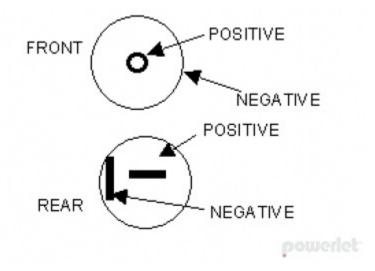
Powersport Standard Connectors are fully DIN ISO standard compliant. Rated for 15 amps.
