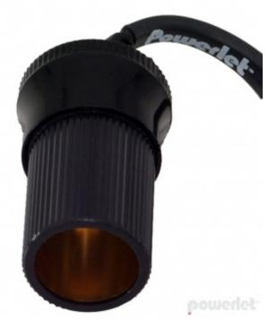
Powerlet only uses 21mm for a tight fit, 22.2mm have loose fit and may disconnect with vibration.
