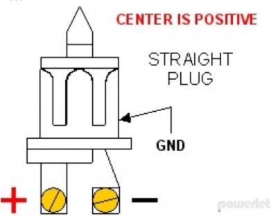
Powersport Standard Connectors are fully DIN ISO standard compliant. Rated for 15 amps.
