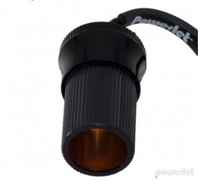
Powerlet only uses 21mm for a tight fit, 22.2mm have loose fit and may disconnect with vibration.
