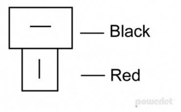
Uses 1/4" spade terminals in a "T" configuration. Used by Powrelet and some vehicle manufacturers like Victory, Aprilia and Triumph.
