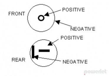
Powersport Standard Connectors are fully DIN ISO standard compliant. Rated for 15 amps.
