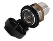
Powerlet sockets are smaller than a cigarette socket, vibration proof, and can handle high current loads. Six of the eleven major vehicle manufacturers use 'Compatible With Powerlet' connectors instead of cigarette sockets. The Powerlet Equipped System is designed around this connector. The Powerlet connector is also a nonproprietary DIN/ISO open standard that is factory installed on many brands of vehicles.
