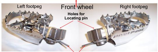
Spring legs lean against the motorcycle frame and are compressed when pegs are moved into position and locating pins are inserted. Trim to length if required.
