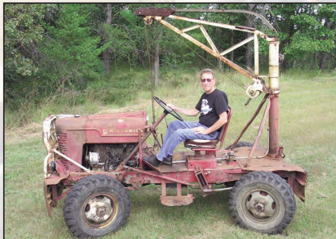
Wayne's Jitney - A WWII Dodge Power Wagon pickup truck with two front ends. Built by Wayne's Uncle Eddy in 1948. Note the adjustable rear steering.
