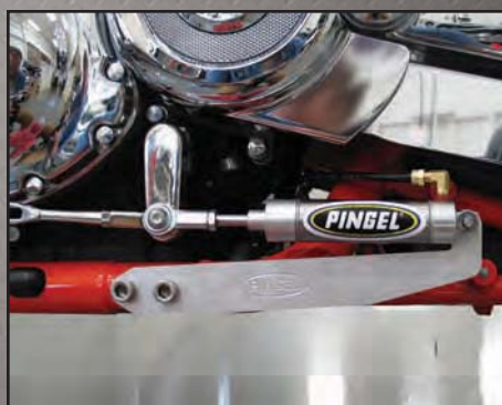
711V Super Electric over Air Shifter Kit installed on a Harley-Davidson V-Rod using a Pingel air shifter mounting bracket, part #62105
