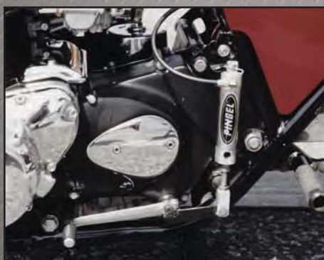
702 Super Air Shifter Kit installed on a Kawasaki KZ
