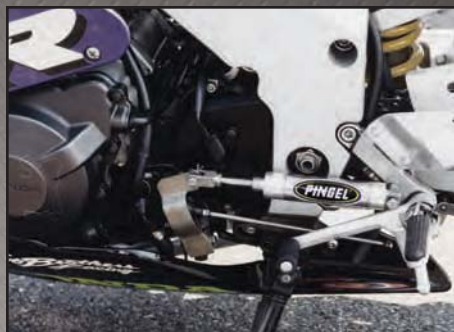
708 Super Electric over Air Shifter Kit installed on a Honda CBR
