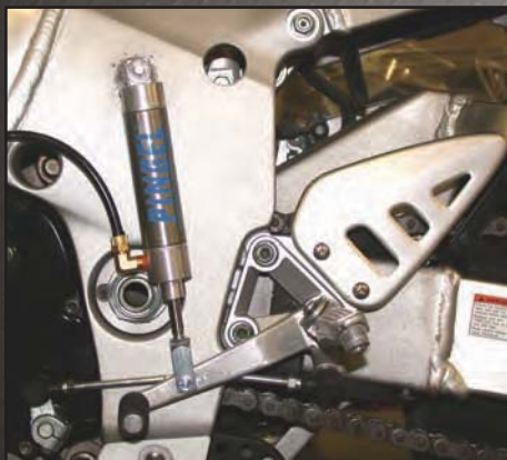
711 Super Electric over Air Shifter Kit installed on a Suzuki GSXR
