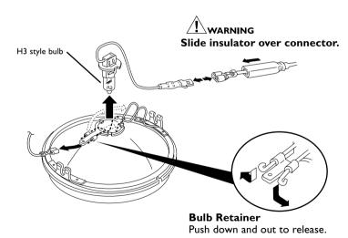
When service is complete reverse steps to assemble lamp. Make sure to not pinch wire while assembling.
