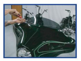
3. Place the PM windscreen trim onto the fairing and install the supplied 1/4" button head center bolt and leave loose. Install the outer 2 bolts and torque to 20-30 in-lbs.
