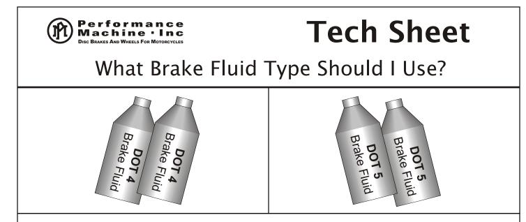
Beginning in 2006, HD switched to a DOT 4 Brake Fluid. DOT 4 fluid (as well as DOT 3) is glycol based while DOT 5 is silicone based. DOT 4 is tolerant to higher temperatures, but is more susceptible to moisture contamination, as well as corrosive to paint. DOT 5 is not as tolerant to high temps, but will generally not hurt paint and is NOT recommended for ABS braking systems.
